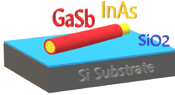
Figure 14.3: A schematic of a partially etched InAs/GaSb NW placed on T-Gate substrate that is covered with 150 nm of SiO 2 . This SiO 2 layer serves as a BG dielectric.
